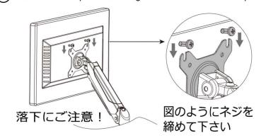
3) Install the lower two screws and fasten the upper two screws.
